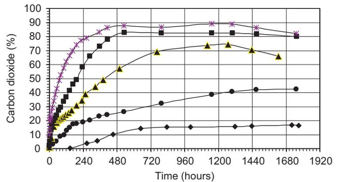
Fig. 6. Levels of CO<sub>2</sub> at moisture contents of 14%, 16%, 18%, 20% and 22% and 30 °C throughout the tested hermetic storage period (◆, m.c. 14%; ●, m.c. 16%; ▲, m.c. 18%; ■, m.c. 20%; and \*- , m.c. 22%).
