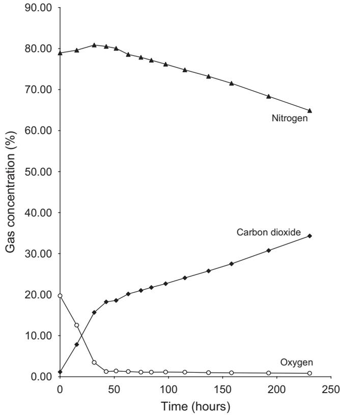
Fig. 3. Gas changes in corn at 18% moisture content during hermetic storage.
