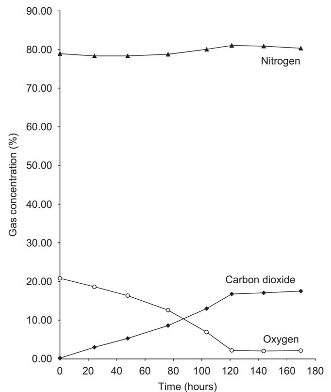
Fig. 2. Gas changes in corn at 16% moisture content during hermetic storage.
