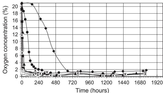
Fig. 7. Levels of  $\text{O}_2$  at moisture contents of 14%, 16%, 18%, 20% and 22% and  $30^\circ\text{C}$  throughout the tested hermetic storage period ( $\blacklozenge$ , m.c. 14%;  $\bullet$ , m.c. 16%;  $\blacktriangle$ , m.c. 18%;  $\blacksquare$ , m.c. 20%; and  $\ast$ , m.c. 22%).
