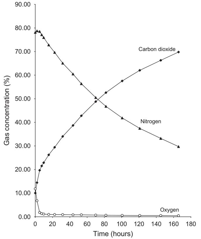
Fig. 5. Gas changes in corn at 22% moisture content during hermetic storage.
