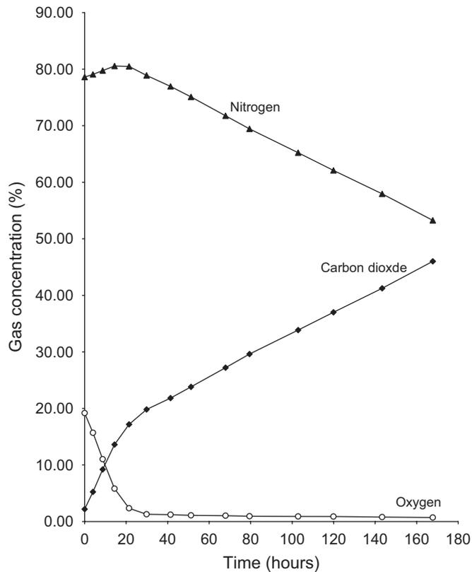
Fig. 4. Gas changes in corn at 20% moisture content during hermetic storage.
