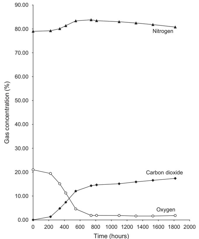
Fig. 1. Gas changes in corn at 14% moisture content during hermetic storage.
